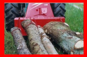
The dozerblade is designed with additional height and a wide log-towing bar to handle even the largest logs.
