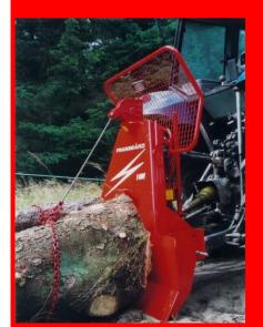
Protective screen guards the tractor in case a cable should **break**.
